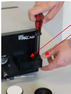
Fig. 33: Loosening the M3 cross-head screws
