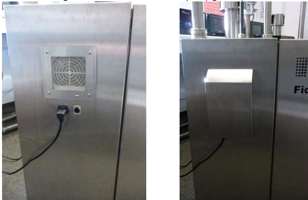
Fig. 22 A+B: Power connection of the weather-protective housing
