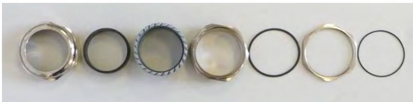
Fig. 8: Components of the fixing of the weather station tube
