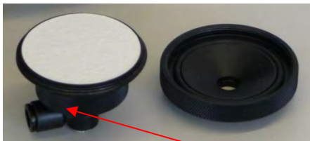
Fig. 30 A: Setup of the filter holder
