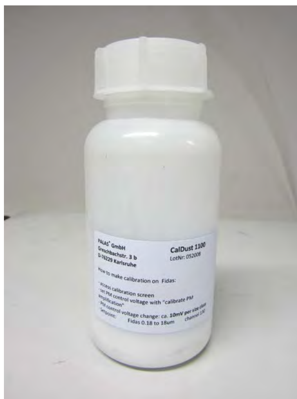
Figure 19: CalDust 1100 for verification / calibration of sensitivity
