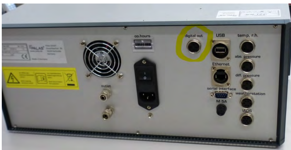
Figure 129: Rear side of instrument with additional port (marked in yellow)
