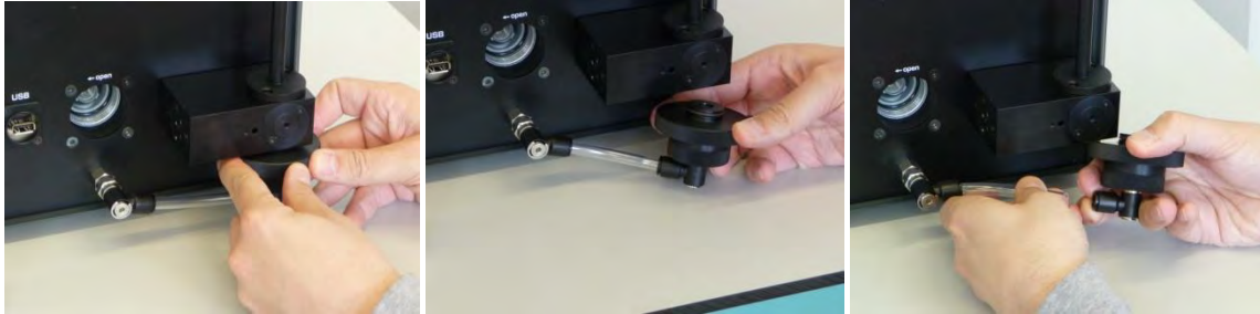
Fig. 29 A-C: Removing the filter holder
