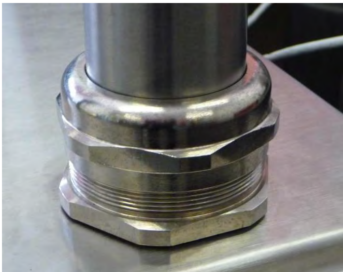
Fig. 9: Fixing of the weather station tube
