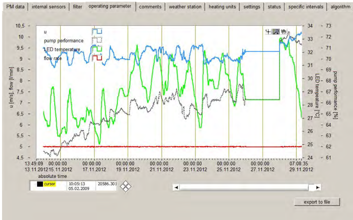
Figure 16: Tab “operating parameter” showing particle velocity, pump performance, LED temperature and flow rate
