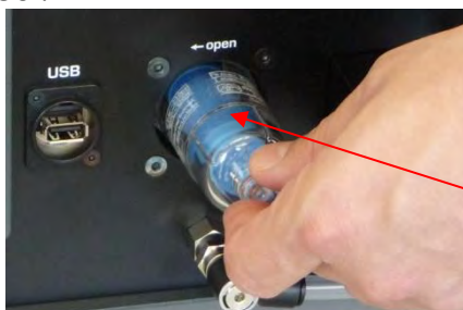
Fig. 37: Removing the protection cap
