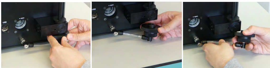
Fig. 32 A-C: Removing the filter holder
