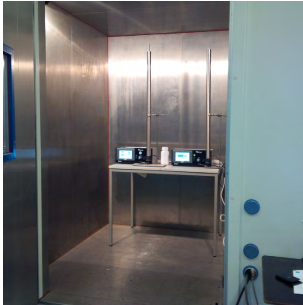
Figure 128: Candidates Fidas® 200 in climate chamber
