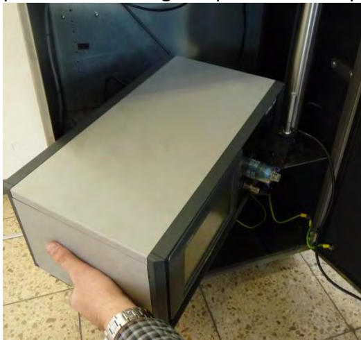
Fig. 15: Insertion of the Fidas® control unit
