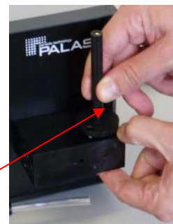
Fig. 34: Removing the aerosol guiding tube
