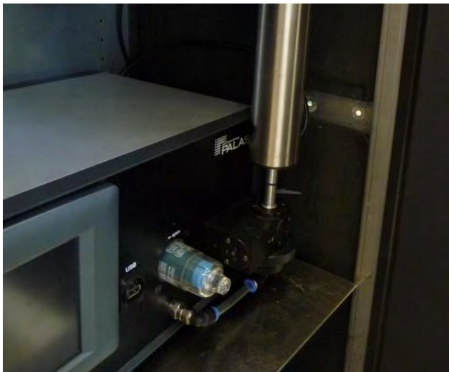
Fig. 17: Connection of the sampling tube with the sampling inlet tube and the control unit
