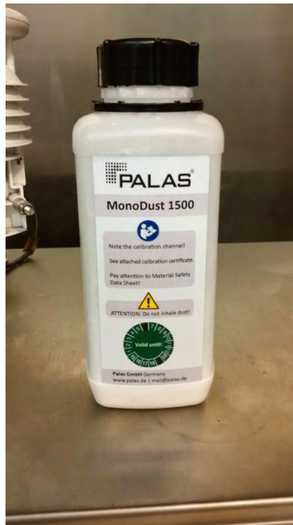
Figure 22: MonoDust 1500 for verifying/calibrating the sensitivity
