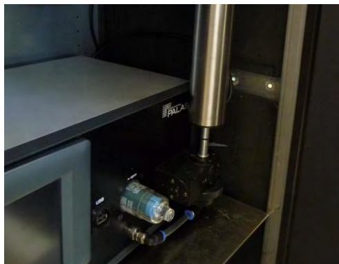
Fig. 31: Connection of the aerosol inlet with the IADS
