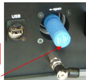
Fig. 38: Filter without protection cap
