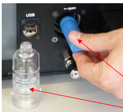
Fig. 37: Removing the protection cap
